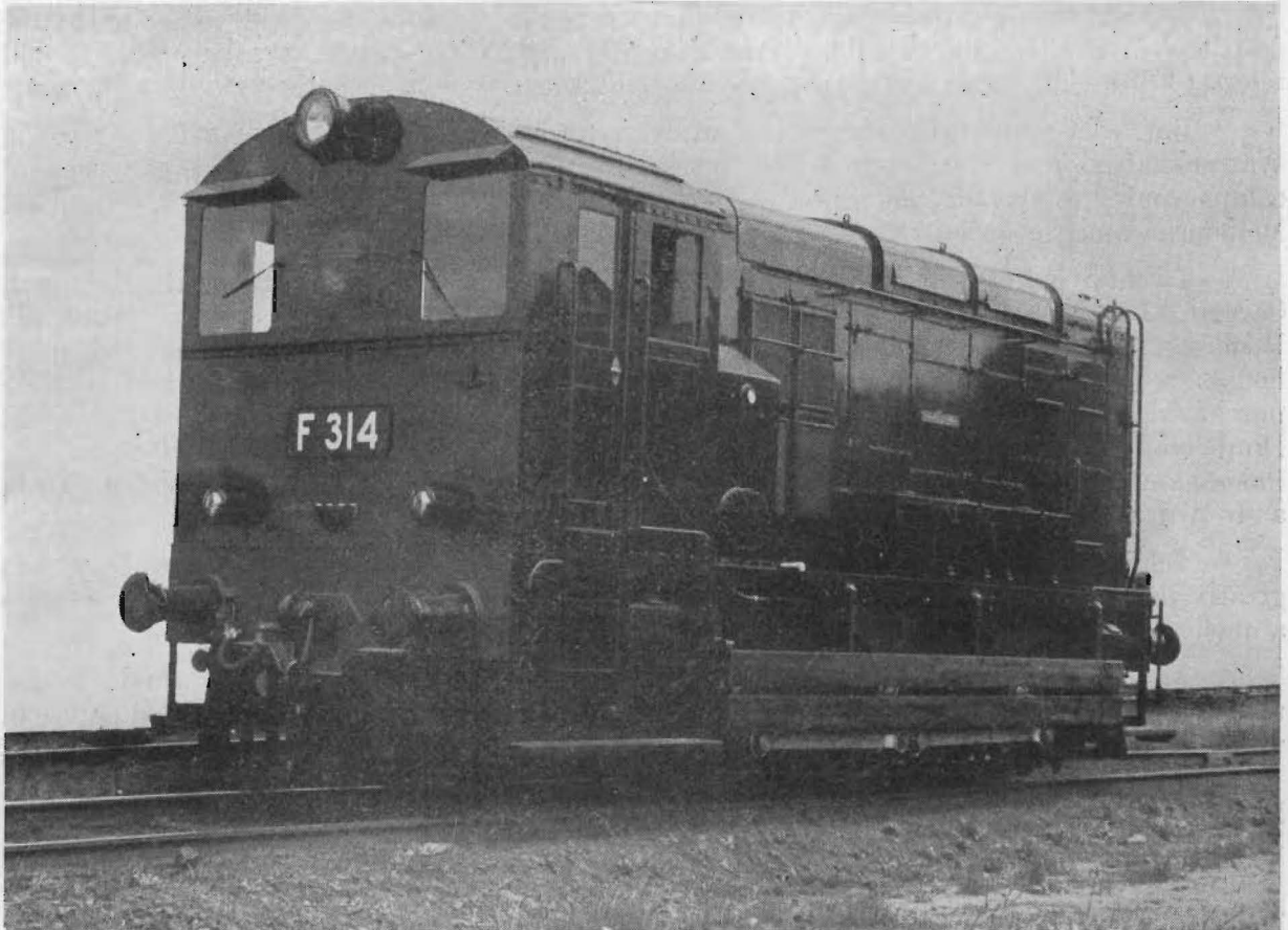
Diesel-Electric Shunting Locomotive.
